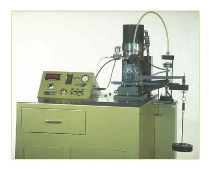
Manufactured by Falex Corporation since 1982, the Falex Timken Test Rig is supplied as a complete system to conduct ASTM Standard Test Methods D2509 and D2782.
